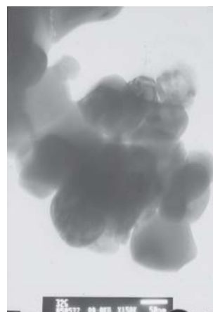
Fig. 3 TEM image of the n -TiC in carbon cages (30 nm, 3 mass% of C matrix)
